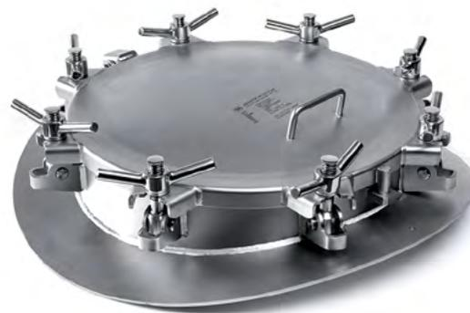
Stainless steel EN 1.4301/7 (AISI 304/L) o EN 1.4401/4 (AISI 316/L); 4-6-8 point fastening with screw and handnut in stainless steel; neckring thickness 8 mm and standard height 125 mm adaptable to various sizes with compensating ring; cover thickness 4 mm. Gasket supplied separately depending on the contact fluid. Standard finishing is sandblasting.
